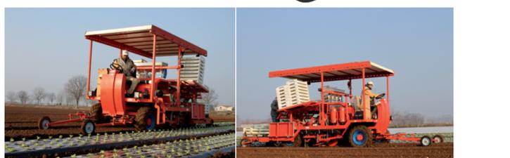
Semi-automatic transplanting machine combined with film-layer for plants in square blocks (side from 3 cm [1.2"] up to 5 cm [2"])
